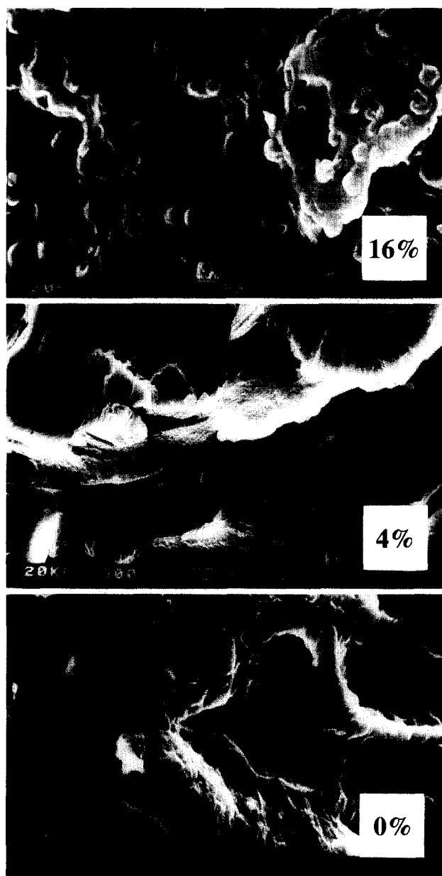
Figure 10 SEMs of room temperature fracture surface of a series of blends of erucamide/i-PP. Their compositions are indicated
